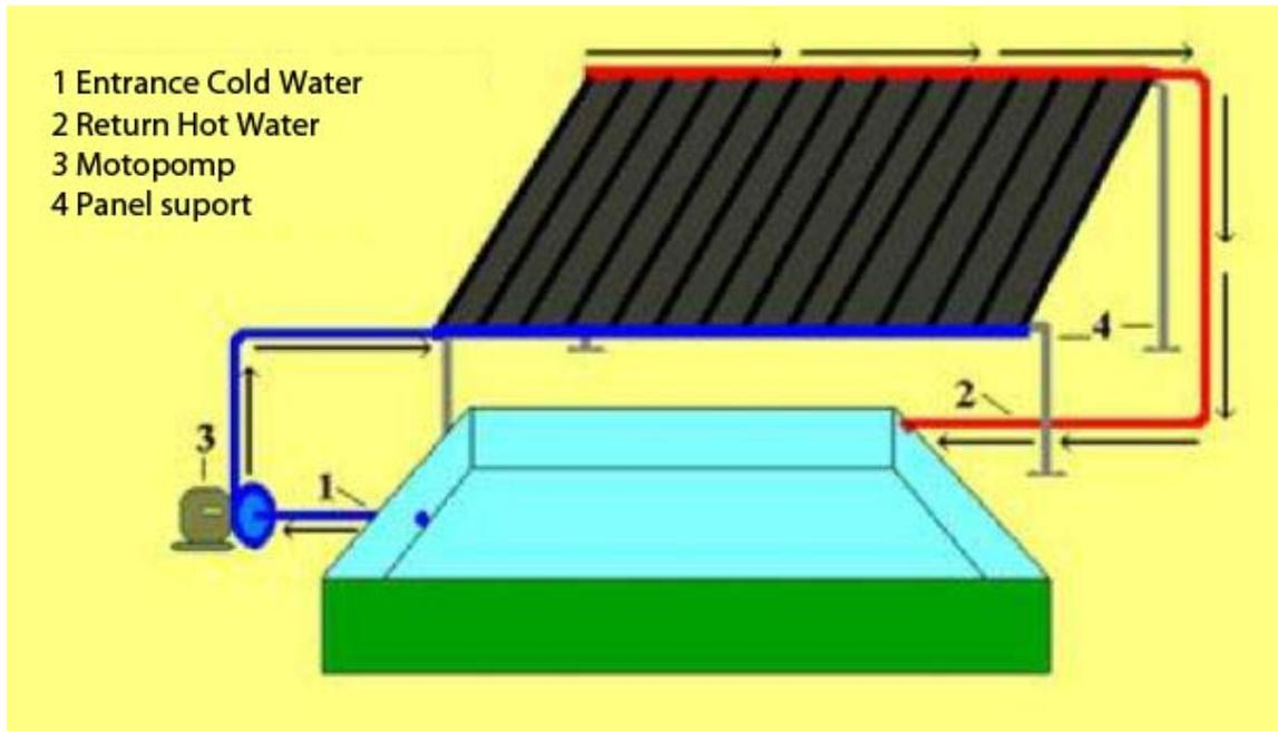
We estimates that to heat water for a shower of one person, a 1m<sup>2</sup> panel would be enough. Materials needed for construction:
